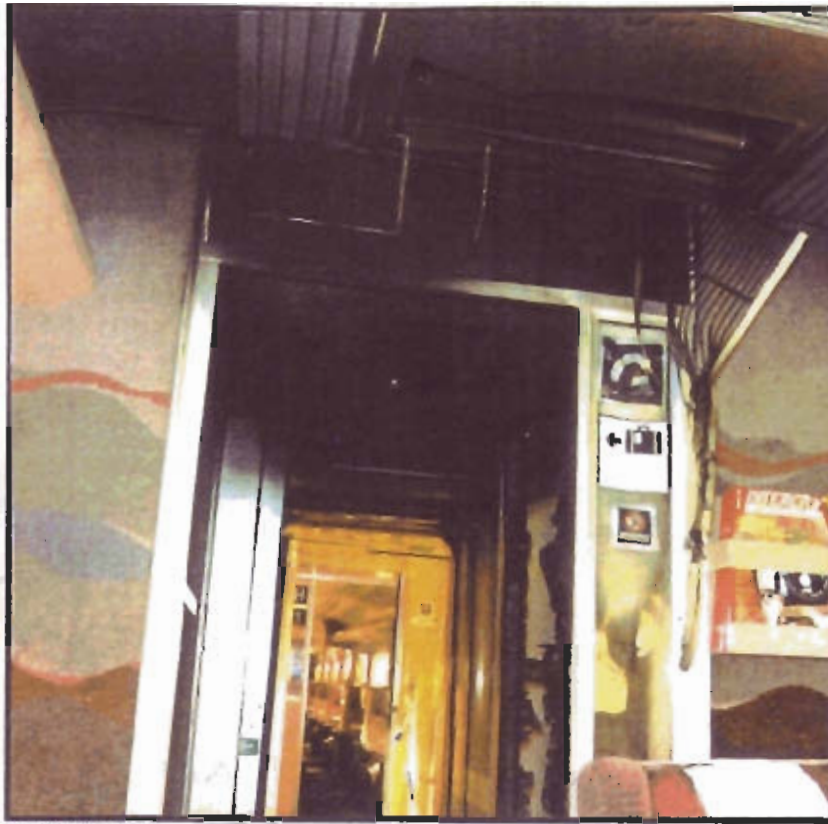
Fig.28 - A view from the front of the compartment of coach G showing damage in the compartment due to the fire in the vestibule
