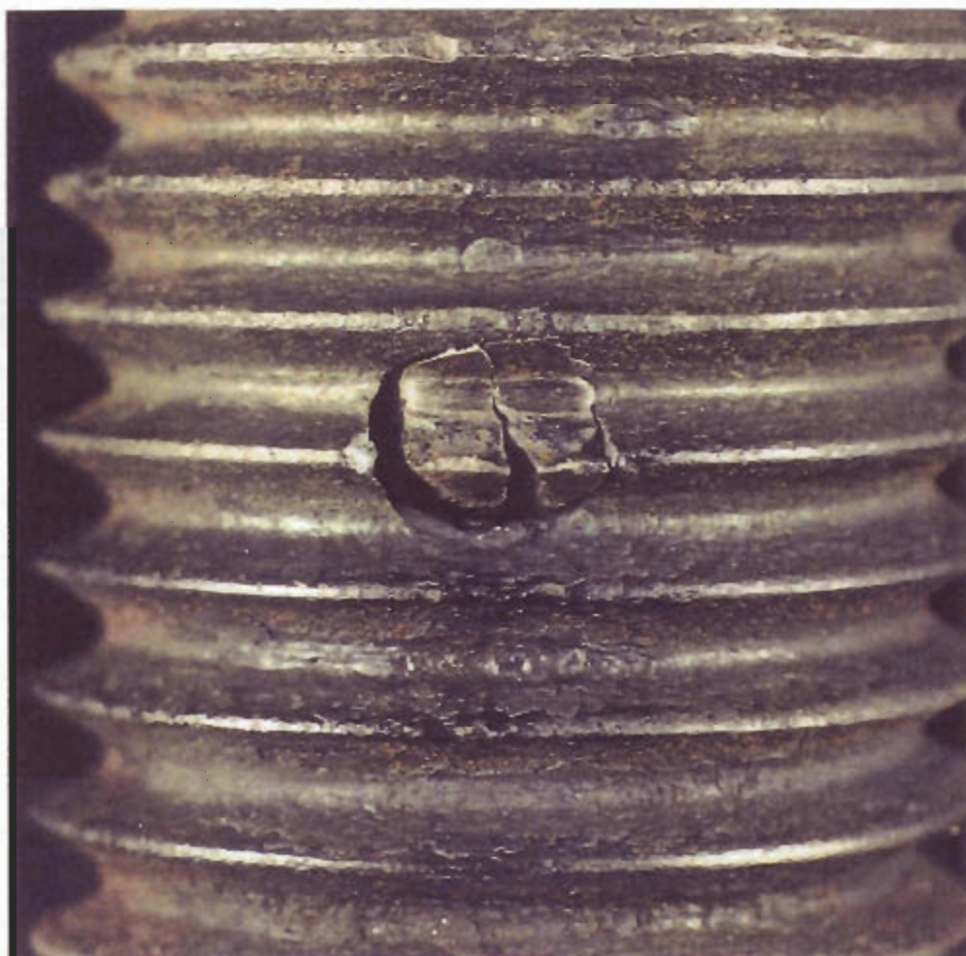
The thread profile in the end of the split pin in the front left hand M24 bolt
