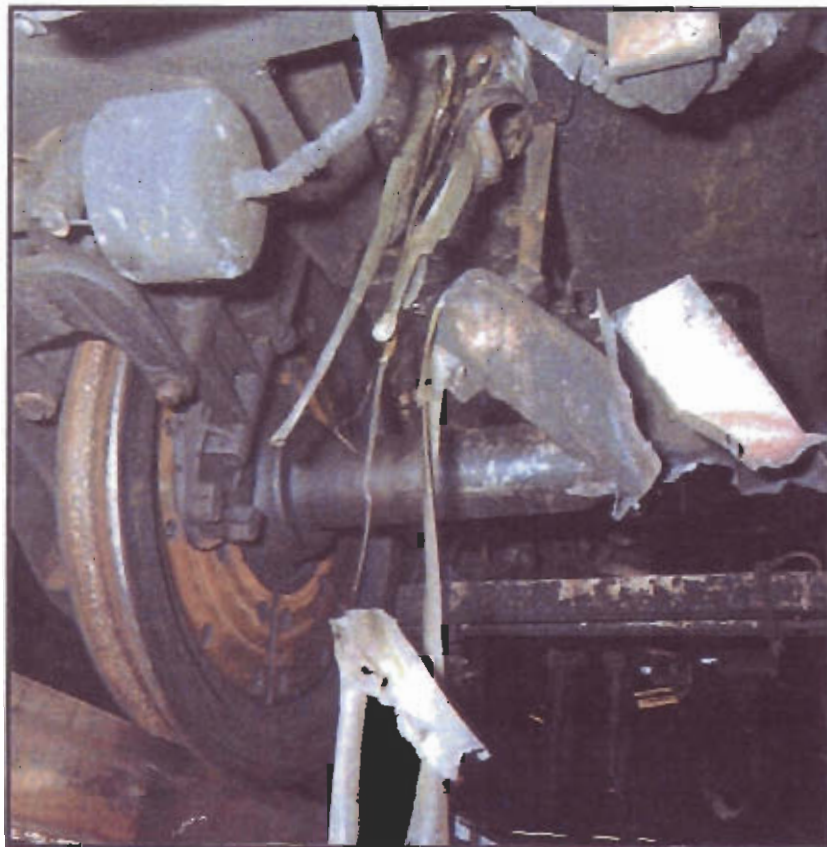
Fig.11b - Close up of fire damage from behind wheel
