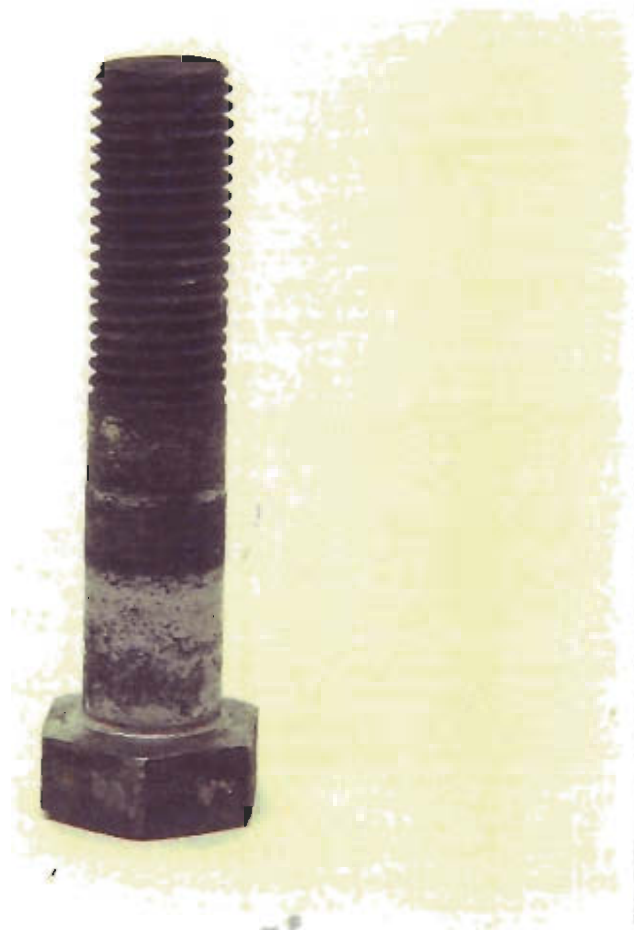
Fig 17 The rear left hand M24 bolt from the rear fuel tank
