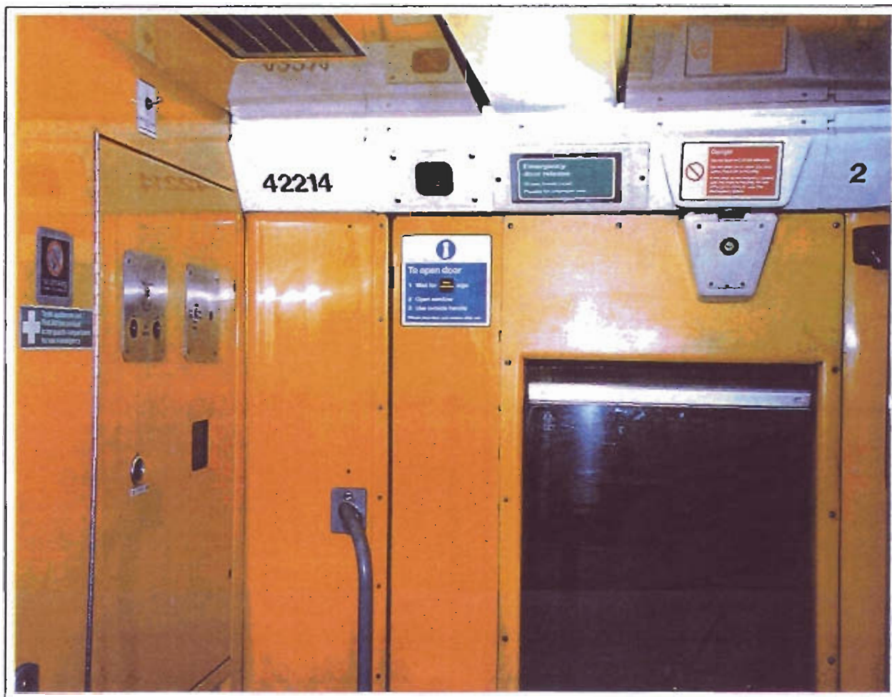
Fig.4 - CDL Systems, typical doorframe arrangement
