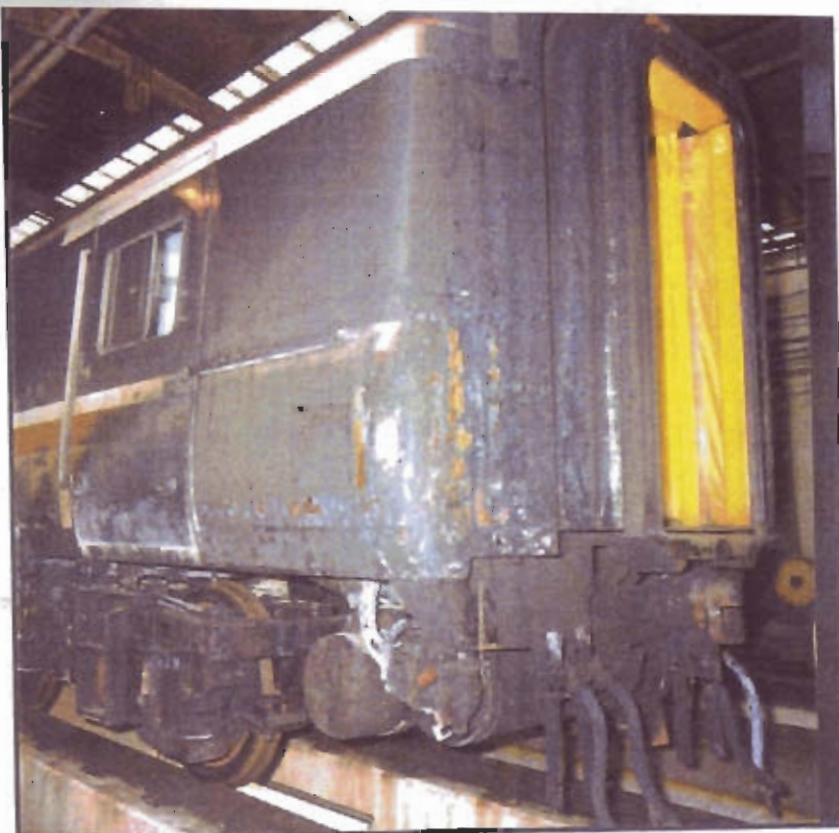
Fig.3a - Rear view of tractor unit after separation APPENDIX A11
