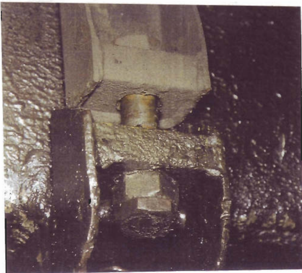
Fig 12 The front left hand M24 bolt on the rear fuel tank
